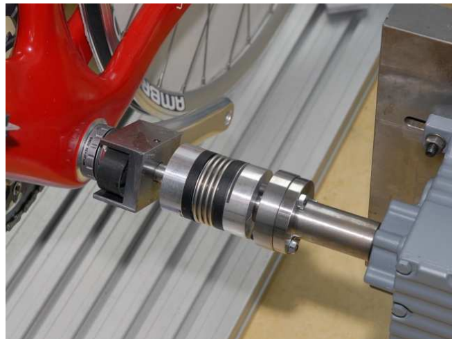
Fig. 2: Drive by means of connection assembly to foot pedal
