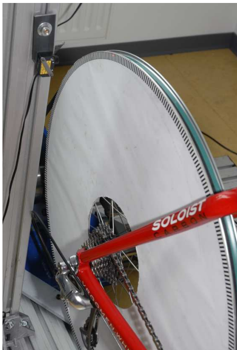
Optical measuring device for speed measurement
