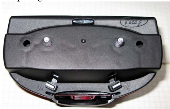
Bolts in 50 mm spacing holes. (Also note positive and ground connection points)
