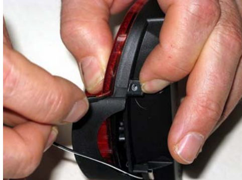
Depress the receiving connector.
