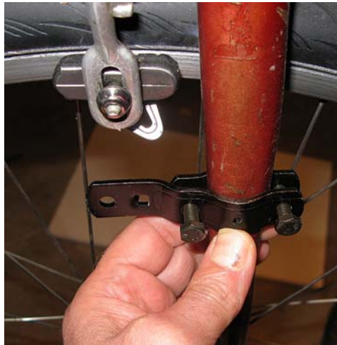
Connect outer half of CS Bracket to inner half.
