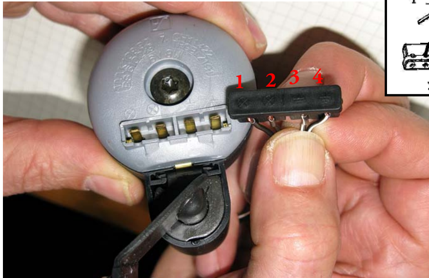
The dynamo and dynamo plug with attached wires. Note: First and third positions are from the wire attached to the headlamp; second and fourth positions are from the wire attached to the rear lamp.
