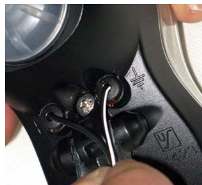
(Left) Fold back exposed wire.
