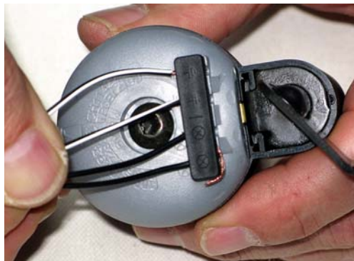
(Left) Press dynamo plug into dynamo. Be sure to match positive-positive and negative-negative. (Right) Trim any excess wire with sharp blade.
