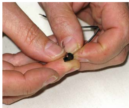
(Left) Fold back exposed wire.
