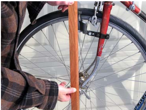
Position dynamo centerline parallel to wheel centerline.
