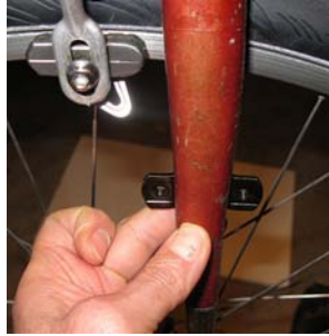
Hold inside half of CS Bracket on inside fork blade.
